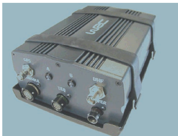
Fitting the DSCP Tracker to the base plate using the rubber straps
